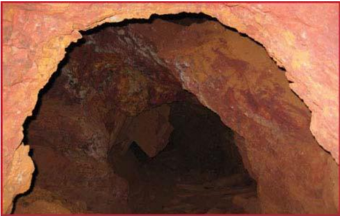
High grade ore pillar and loading chute from the intermediate level of the Cave Mine
